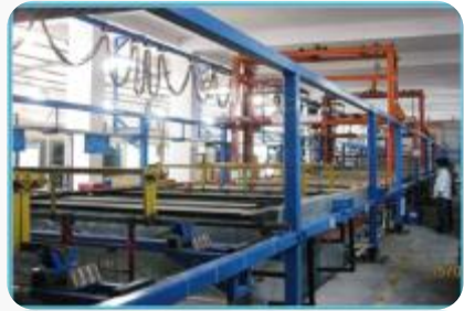
-Automatic Alkaline Zinc Plating.
