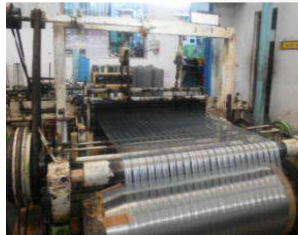
-Wire mesh , Perforation & Expanded Mesh machines -Mesh is used in automobile filter parts
