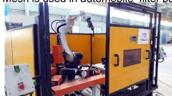
Robotics for Auto Welding of Gear Change Lever Assly
