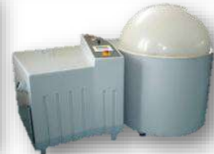
Salt Spray Testing Unit
