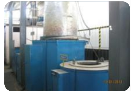
-Liquid Nitriding Process Capacity/Day : 3200 Kgs.
